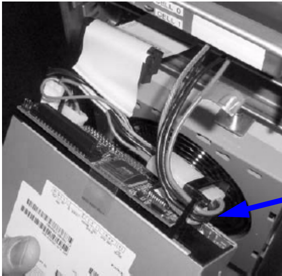
Figure 6-14 Power Cable Connection and Routing
