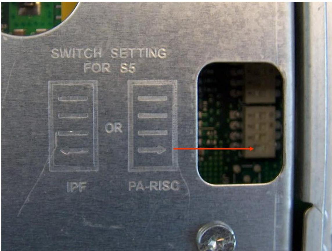
As this picture shows, the switch should be set to the right ("ON") position for "PA-RISC" (e.g. "Mako" PA8800 or "Mako64" PA8900) processors. Set it to the left ("Off") for Itanium2 or MX2 Intel "IPF" processors.
