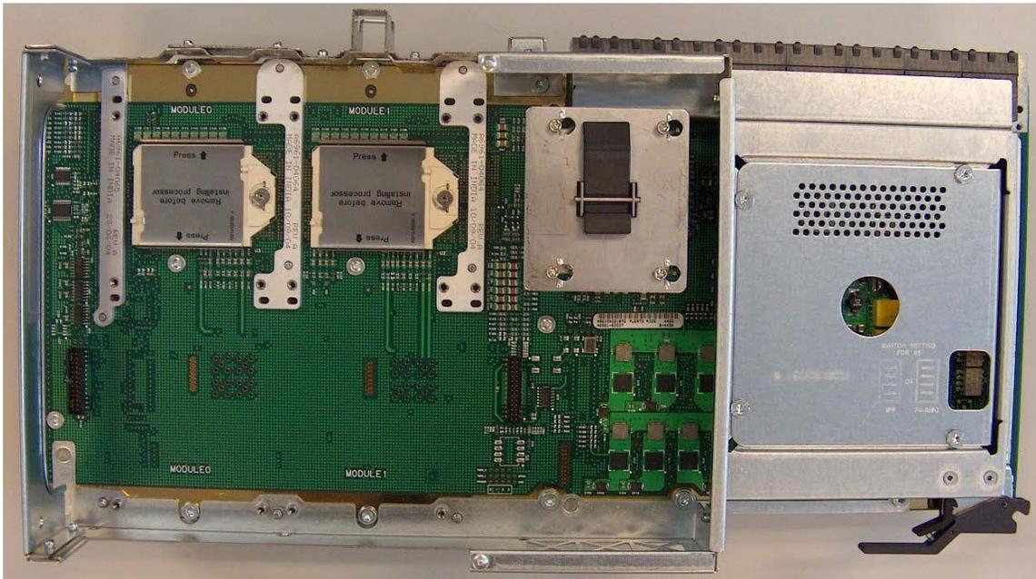
Notice that there SHOULD BE a legend stamped in the sheet metal showing which switch in switch bank S5 (the lowest switch if the CPU Extender is positioned as shown) selects which processor type. A close-up of the sheet metal stamping is shown below:
