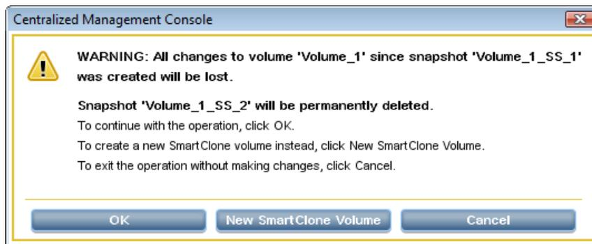
**Figure 9 Rolling back a primary volume if iSCSI sessions are not connected**
