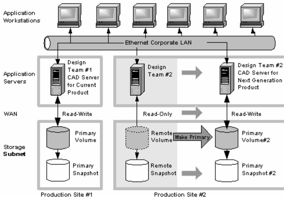
Figure 17 Off-site backup and recovery example configuration
