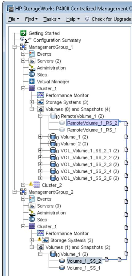
**Figure 4 Remote copy in progress**
