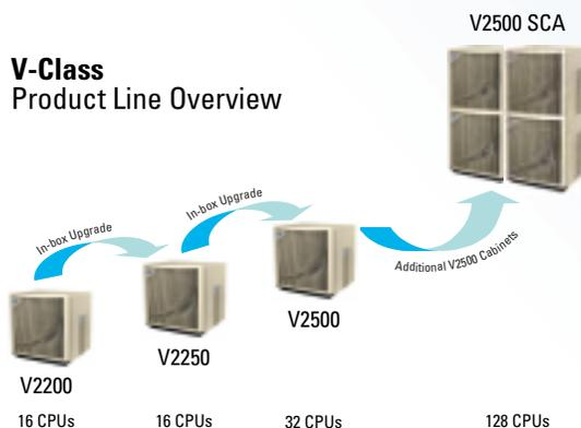
For high-end computing, HP offers three models of V-Class servers. The V2200 is a 200-MHz PA-8200-based 16-way V-Class system. The V2250 is a 240-MHz PA-8200-based 16-way system. Both the V2200 and the V2250 can be upgraded to the 440-MHz PA-8500-based 32-way V2500. Based on HP's unique Scalable Computing Architecture (SCA), the V2500 allows you to scale up to 128 CPUs and 128 GB of memory.
