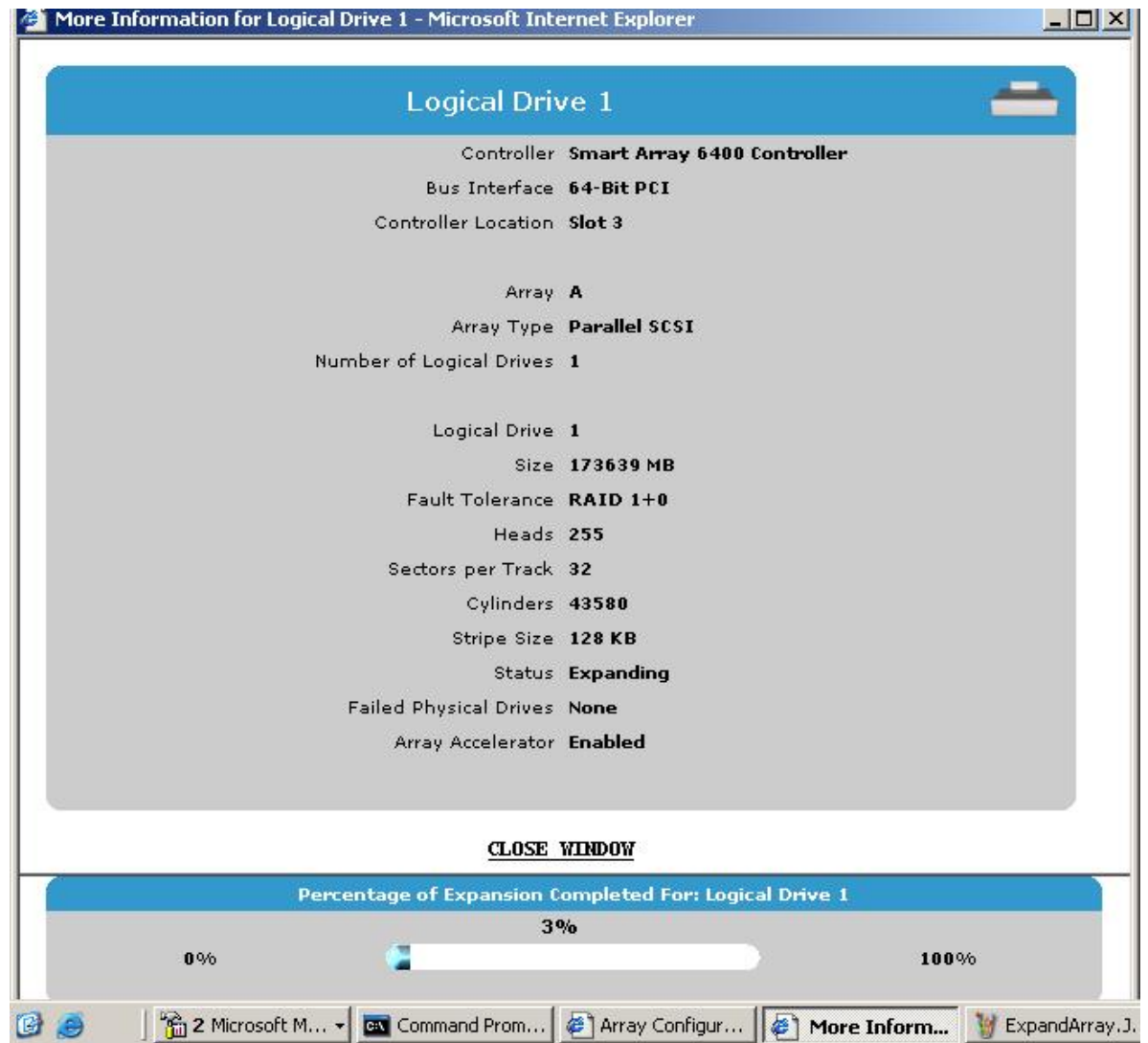
Figure 3. Array Configuration Utility - Expansion Status
