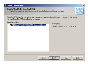
In the example above we can see that we have an Operating System level driver loaded for a Quantum DLT7000 tape drive. The important thing to ensure here is that the red tick-box next to the drive is checked so that ARCserve can control the tape drive.
