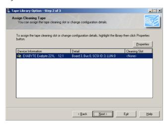
You can click the 'Properties' button to configure options relating to barcode, cleaning slot assignment, automatic drive cleaning, and handling of blank media.
