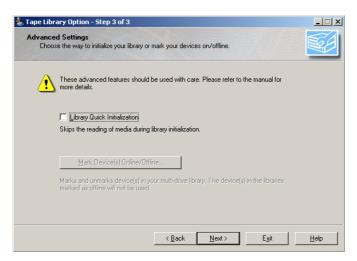
Here, you can configure quick initialization. By default, each time the tape engine is stopped or started, or the tape library door is open/closed whilst the tape engine is operational this will trigger an automatic inventory of all tapes in the library. If you have a large library this may be undesirable.
