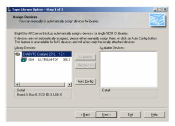
If devices are not automatically assigned in the left-hand pane of the device configuration window as below, then press the 'Auto  $\underline{C}$  onfig' button:
