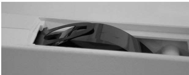
Figure 4 Examples of Tape Cartridge Loop Problems
