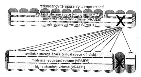
For VRAID1, the data is first copied to unassigned space on different disks from the surviving disk of the mirrored pair. The data is then moved from the surviving disk to the mirrored pairs of the recipient disks.
