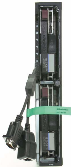
figure 4: the integrated lights-out cable connector inserted into the diagnostic port
