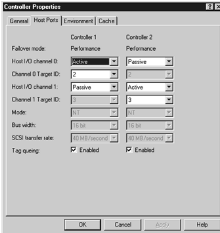
Figure A-4. Host ports configuration screen in the CR3500 configuration utility
