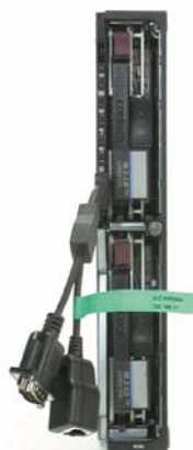
Figure 6a. Diagnostic Cable connected to the BL20p
