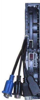
Figure 6b. Local I/O Cable connected to the BL20p G2
