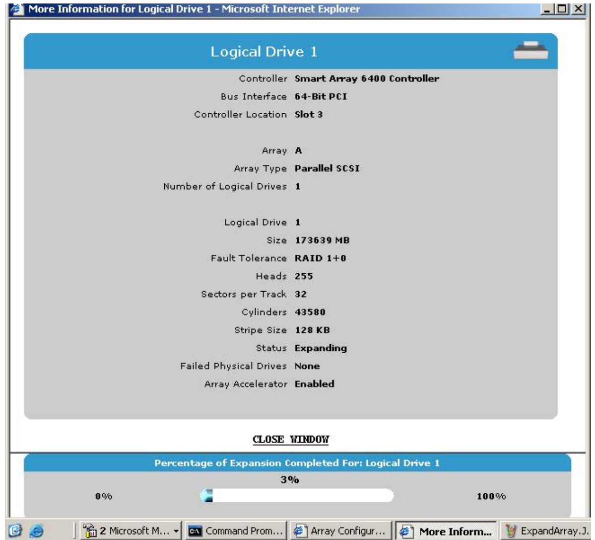
Figure 3. Array Configuration Utility - Expansion Status
