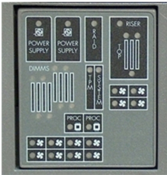
Figure 7 System Insight Display LEDs
