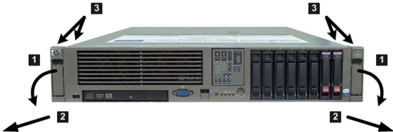
Figure 52 Removing the Front Bezel
