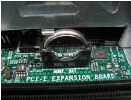
Figure 73 Battery and Battery Socket
