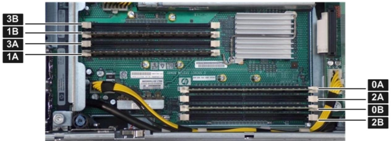
Figure 19 Memory Location and DIMM Slot IDs
