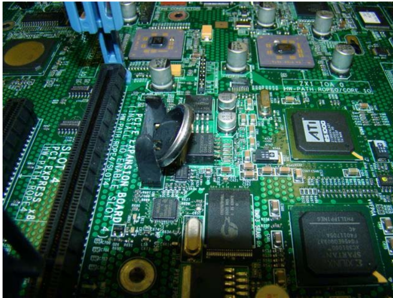
Figure 77 Tilting the Battery Out of or into the Socket
