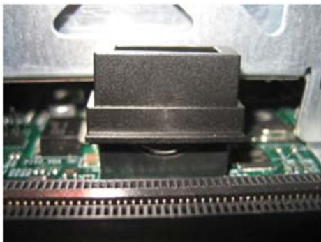
Figure 75 Installed Battery Clip
