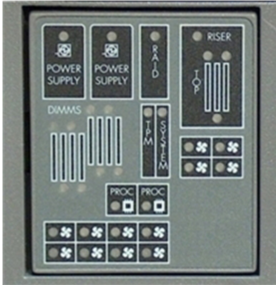
Figure 36 System Insight Display LEDs
