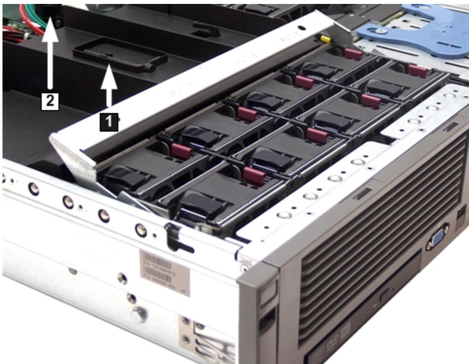
Figure 41 Fan Carrier Handle
