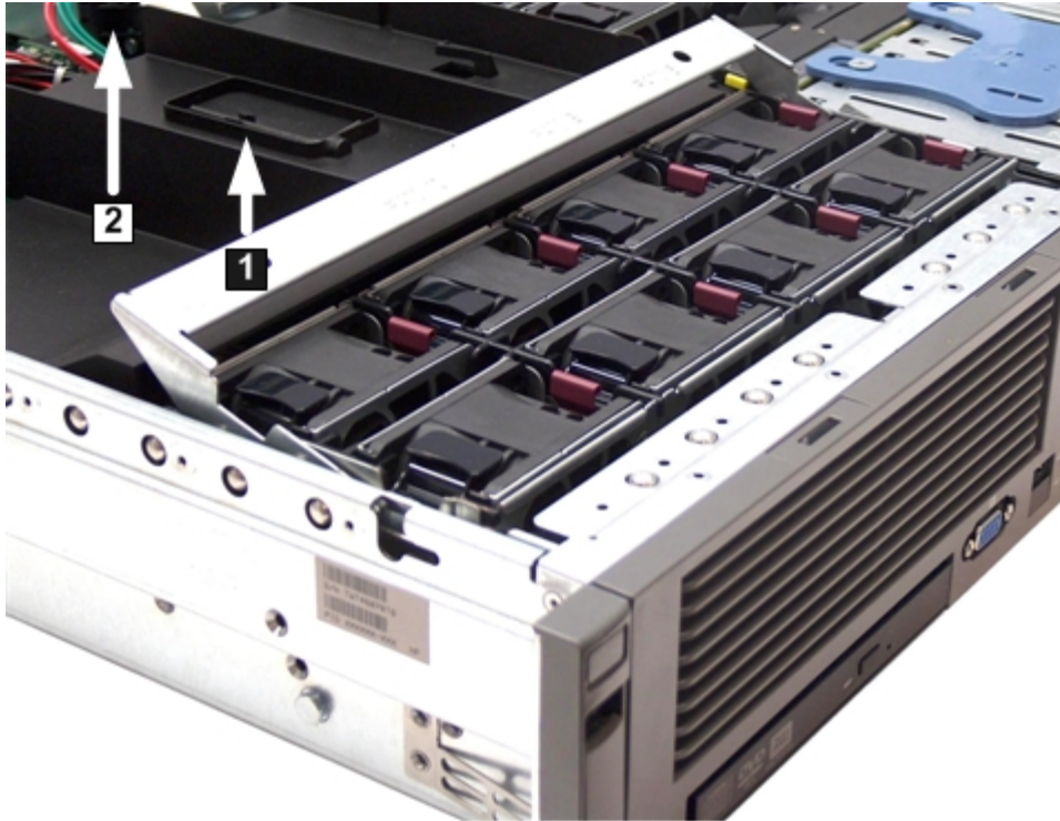
Figure 18 Fan Carrier Handle
