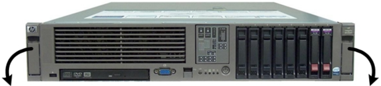
Figure 37 Extending the Server from the Rack
