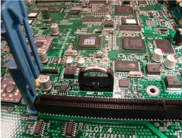
Figure 76 Power Supply Housing Removed For Battery Access
