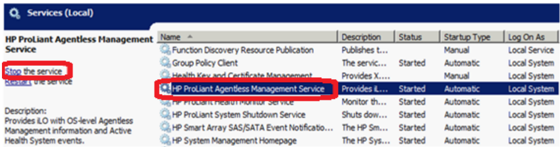
Figure 11: You can start or stop the HP Agentless Management Service in the Windows Services applet.
