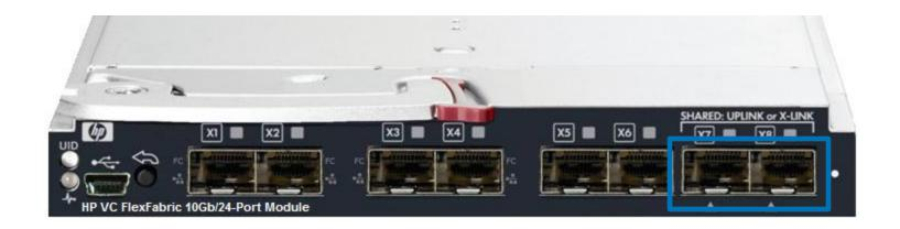
• Port X7 (SFP+) and port X8 (SFP+) are each shared with two internal 10Gb cross-link.
