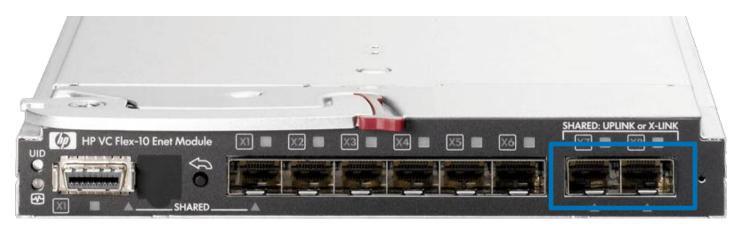
• Port X7 (SFP+) and port X8 (SFP+) are each shared with two internal 10Gb cross-link.
