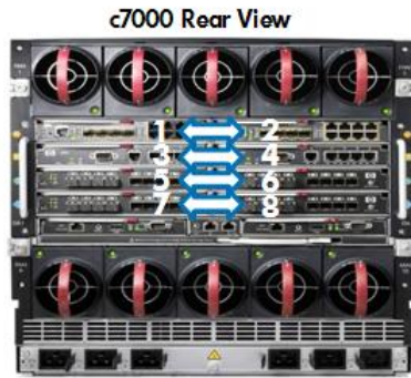
Figure 12. HP BladeSystem c7000 interconnect bay crosslinks as indicated by the arrows
