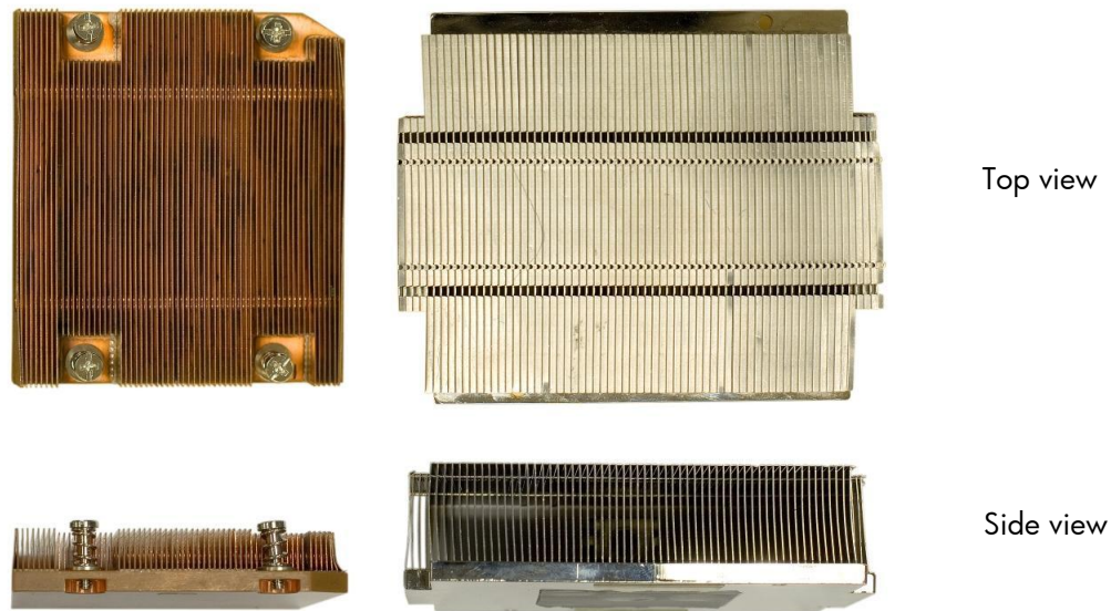
Figure 18. Processor heat sink using fully ducted design (left) versus traditional heat sink in a 1U rack-mount server (right)
