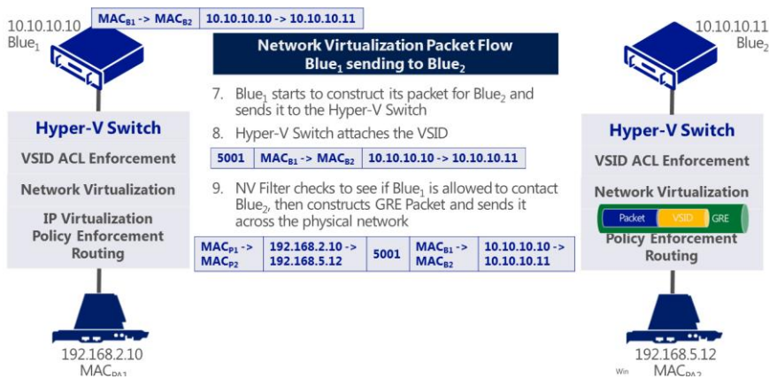
Figure 10: The NV Filter checks to see if Blue1 can contact Blue2. A GRE packet is then constructed and sent across the physical network.
