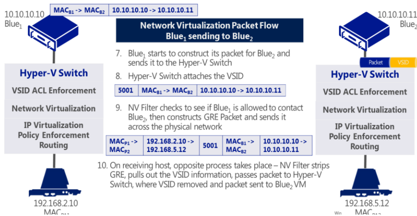
Figure 11: The GRE header is stripped off Blue2. The Hyper-V Switch uses the VSID information to send the packet to the Blue2 virtual machine.
