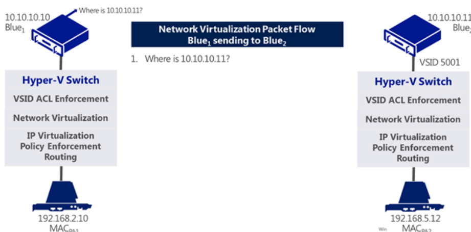
Figure 2: The process of sending a packet from Blue1 to Blue2.
