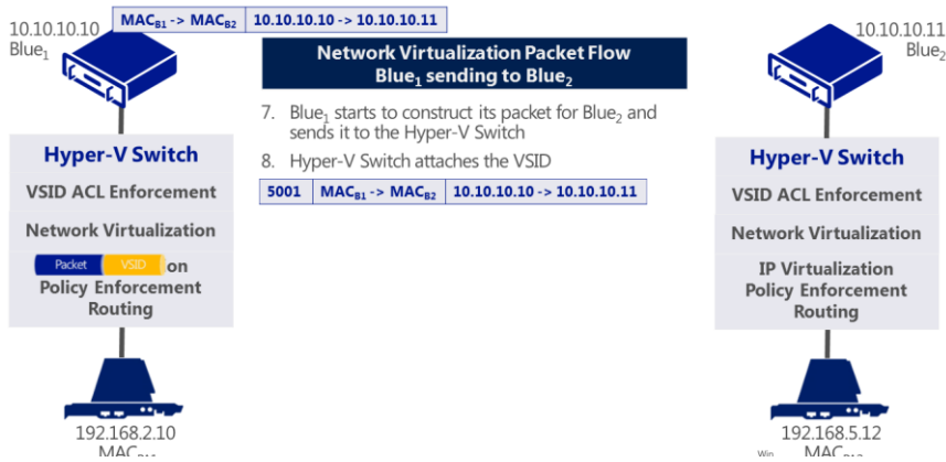
Figure 9: The Hyper-V Switch attaches the VSID header. NVGRE uses the VSID header to route the packet to the correct virtual network.
