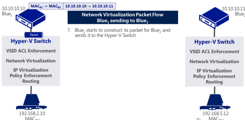
Figure 8: Blue1 constructs the packet for Blue2 and sends it into the Hyper-V Switch.
